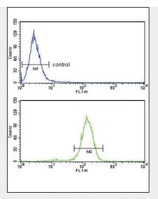
BCL3 Antibody (Center) (Cat. #AP9337c) flow cytometry analysis of Hela cells (bottom histogram) compared to a negative control cell (top histogram).FITC-conjugated goat-anti-rabbit secondary antibodies were used for the analysis.
